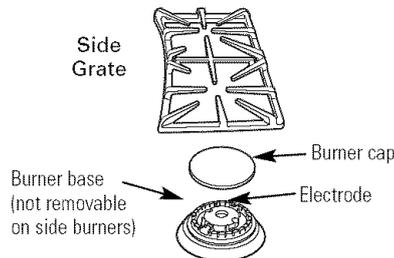
B On models so equipped, assemble the center burner. Make sure that the center griddle sits square and level between the side grates.
