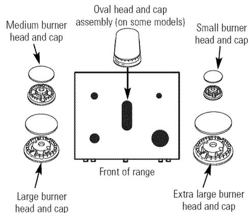
Place the burner caps on the cooktop. Make sure that the caps are placed in the correct locations. There is one small cap, one medium cap, one large cap and one extra large cap.
