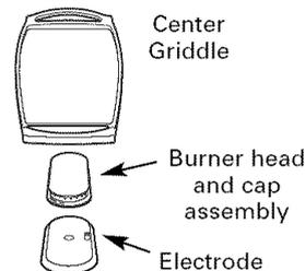
**CAUTION:** Do not operate the burner without all burner parts in place.
