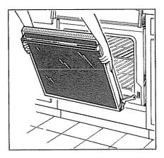
To remove door, open to BROIL position (about 4 inches). Grasp door at sides near top; lift door up and pull out to clear notch in hinge support. Then pull door straight out.
