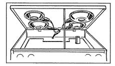
Clean the area under the drip pans often. Built-up soil, especially grease, may catch fire. To make cleaning easier, the entire cooktop may be lifted up and held up by a supporting rod that can be stored under the cooktop.
