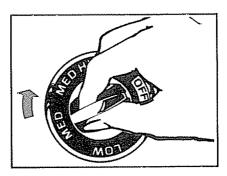
**Step 2:** Turn either clockwise or counterclockwise to desired heat setting.
