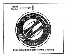
IMPORTANT: For normal cooking, line up the desired temperature (marked on the outer edge of the control knob) with the index marker located immediately above the control.
