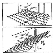
TO REMOVE shelf from the oven, pull it forward until it stops; then tilt up the front edge and pull the shelf all the way out. Be certain the shelf is cool before touching.
