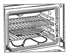
The oven has four shelf supports—A (bottom), B, C and D (top). Shelf positions for cooking food are suggested on Baking, Roasting and Broiling pages.
