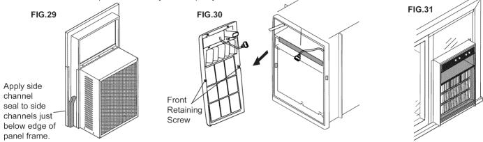
**Drill two 9/64" diameter pilot holes** in the top window jamb in line with the partially plugged holes in the panel frame. Secure the panel frame to the window jamb with two #8-32 x 3/4" self-threading screws. If additional holding is necessary, two screws may be used on the sides of the panel frame as well.
