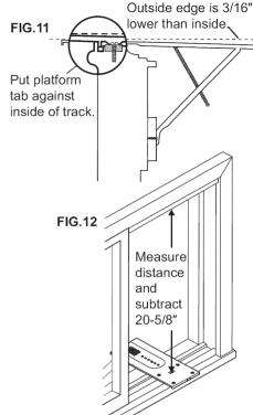
19 Slide inner window sash firmly against side of the cabinet. Make sure not to peel the seal strips from the window track and cabinet side channels. If the panel frame does not fit snugly to the inner window sash, secure the panel frame to the sash with #8 x 3/4" self-threading screws. Use the partially plugged holes in the panel frame. Drill 1/8" pilot holes for the screws.
