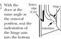
into the bottom of the slot.
