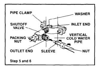
6. Slip compression nut and compression sleeve on copper tubing as shown in diagram. Insert end of tubing into outlet end squarely as far as it will go. Screw compression nut to outlet end with adjustable wrench. Do not overtighten. Turn ON main water supply and flush out tubing until water is clear. Turn OFF shutoff
