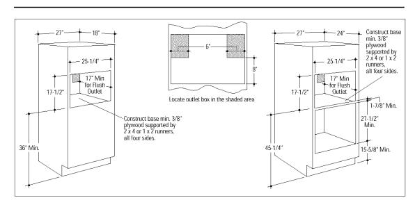
Installation Options Monogram built-in ovens can be inset into the cabinetry. In this installation the microwave is recessed and flush with the front surface of the cabinet.
