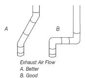
Allow as much room as possible when using elbows or making turns. Bend vent gradually to avoid kinking.
