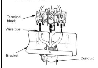
Wire used, location and enclosure of splices, etc., must conform to good wiring practices and local codes.
