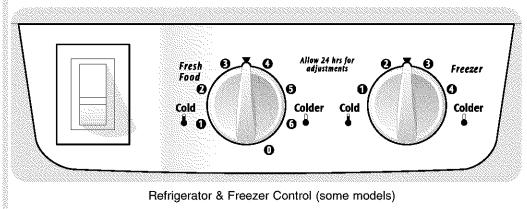
\* IMPORTANT: Turning the refrigerator temperature control to "0" turns off the compressor, but does not disconnect the power to the light bulb and other electrical components. To turn off power to your refrigerator, you must unplug the power cord from the wall outlet.
