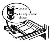
The shutter for the bottom (oven) burner is near the back wall behind the storage drawer or warming drawer. Remove the drawer. See the *Care and cleaning of the range* section.
