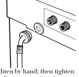
outlet of the water valve. Tighten by hand; then tighten another 2/3 turn with pliers. **Do not crossthread or over-tighten these connections.**
