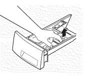
Remove the inserts from the bleach and fabric softener compartments. Rinse the inserts and the drawer with hot water to remove traces of accumulated laundry products.
