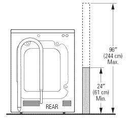
**NOTE:** The drain hose attached to the washer can reach a 90" (229 cm) high standpipe. For a higher standpipe, contact an authorized parts distributor. If the drain is less than 24" (61 cm), install a siphon break kit, available at your local hardware store.
