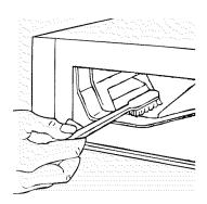
■ To clean the drawer opening, use a small brush to clean the recess. Remove all residue from the upper and lower parts of the recess.
