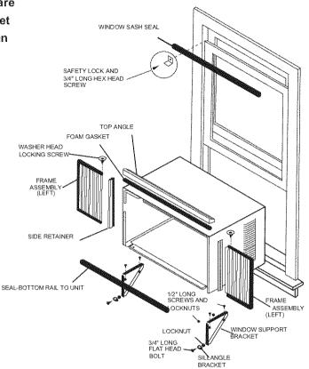
Check your storm windows - if you storm window frame does not allow the clearance required, correct by adding a piece of wood as shown in FIG.2, or by removing storm window while room air conditioner is being installed. (continued)
