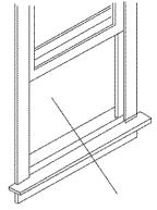
2. Place cabinet in window with bottom stool angle firmly scated over window stool as shown. Bring window down temporarily behind top angle to hold cabinet in place.
