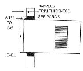
4. Secure bottom rail to wood frame with two large wood screws 1"(2.5 cm)long using the two holes in the bottom of the channel resting on frame.(See FIG.2 following)
