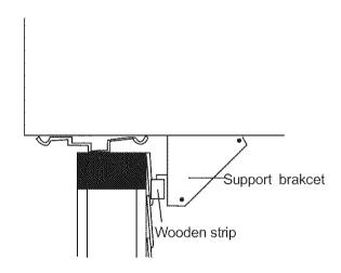
Screw or nail cabinet wooden frame using shims if frame is oversized, to eliminate distortion. Remember to maintain proper slope as described in Step 3.
