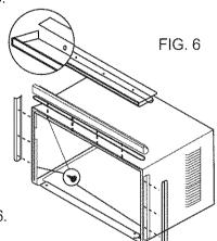
Install top angle and side retainers to cabinet as shown in FIG. 6.
