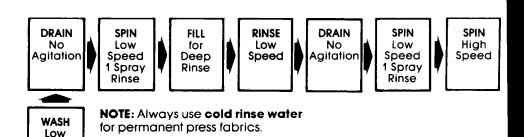
\* IMPORTANT: THE WASHER WILL PAUSE BRIEFLY THROUGHOUT EACH CYCLE. These pauses are normal. They allow for the reversing of the motor, normal washer operation, and the cool down portion of the PERMANENT PRESS Cycle.
