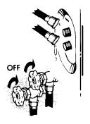
Shut off both water faucets. Disconnect and drain water inlet hoses.
