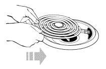
**4.** When the terminal is pushed into the receptacle as far as it will go, push down the edge of the coil element opposite the receptacle.
