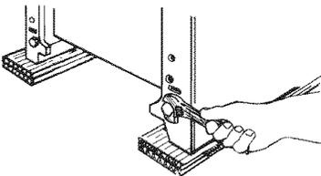
5. Use an adjustable wrench to loosen the leveling legs 1-1/2 turns.
