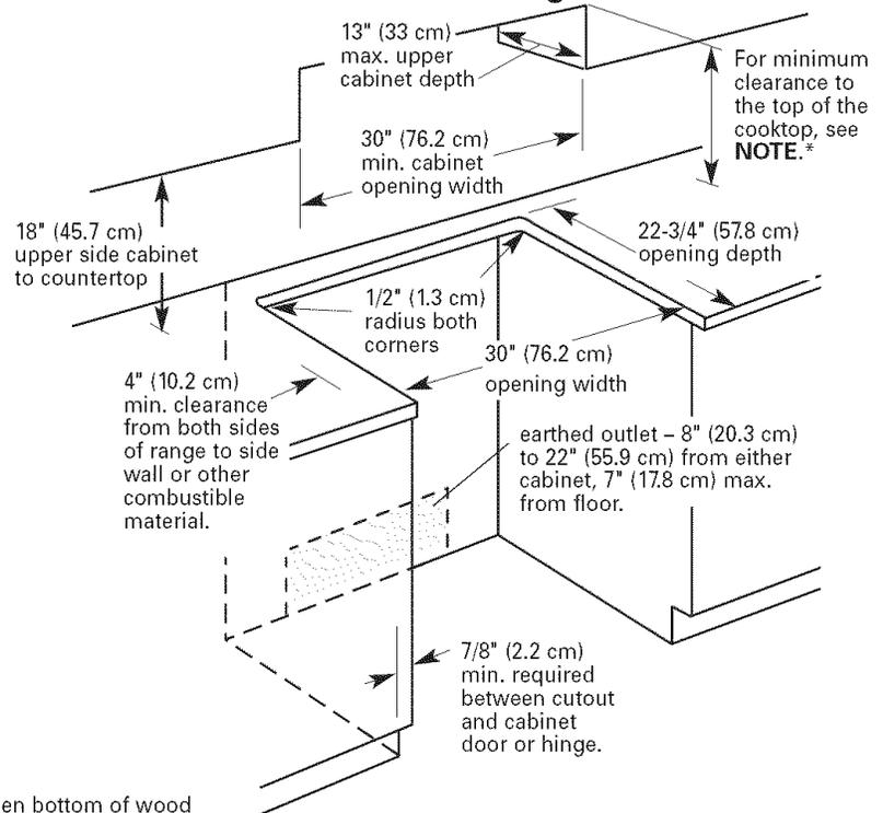
\* NOTE: 24" (61 cm) min. when bottom of wood or metal cabinet is protected by not less than 1/4" (0.64 cm) flame retardant millboard covered with not less than No. 28 MSG sheet steel, 0.015" (0.4 mm) stainless steel, 0.024" (0.6 mm) aluminum or 0.020" (0.5 mm) copper.
