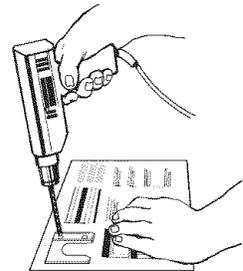
9. Line up holes in anti-tip bracket with holes in floor. Use the screws provided to fasten anti-tip bracket to floor.
