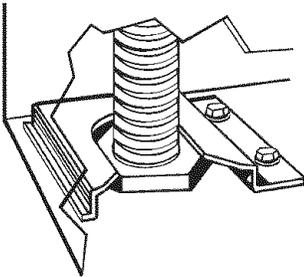
**14.** Place rack in oven. Place level on rack, first side to side; then front to back. If the range is not level, pull range forward until the rear leveling leg is removed from the anti-tip bracket. Adjust the leveling legs up or down. Then slide range back into position. Check that leveling leg is engaged in anti-tip bracket.
