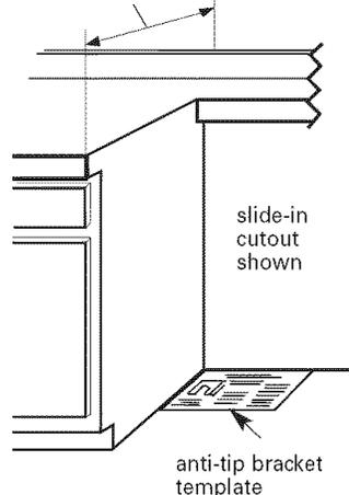
If countertop is not flush to the side of cabinet opening, align the left side of the template to allow for the countertop overhang. Tape the range anti-tip bracket template in place.
