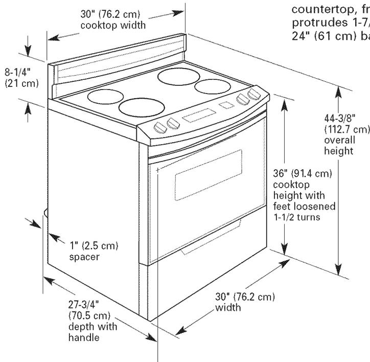
When installed in a 24" (61 cm) base cabinet with 25" (63.5 cm) countertop, front of oven door protrudes 1-7/8" (4.8 cm) beyond 24" (61 cm) base cabinet.
