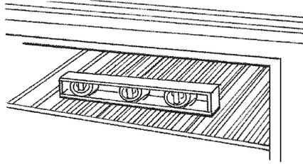
**15.** Insert storage drawer into slide rails on sides of drawer opening. Lift front of drawer slightly and push firmly to close drawer.
