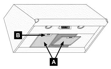
2. While pushing back on the release lever, lower the filter out of the hood. On hoods with more than one filter, remove and clean all of the filters.
