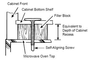
**5.** Insert 1 self-aligning screws through outer top cabinet holes. Turn two full turns on each screw.
