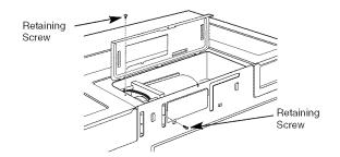
**3.** Carefully slide the blower motor toward the right, and lift it partially out of the opening. **Note:** The blower wires are long enough to allow flexible handling while performing these steps. Disconnect the wires if necessary for additional flexibility.
