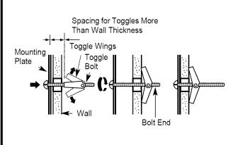
**3.** Place the mounting plate against the wall and insert the toggle wings into the holes on the wall to mount the plate.
