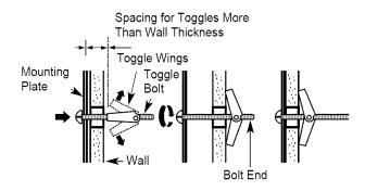
**3.** Place the mounting plate against the wall and insert the toggle wings into the holes on the wall to mount the plate.
