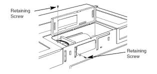
**3.** Carefully slide the blower motor toward the right, and lift it partially out of the opening.
