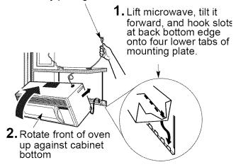
3. Insert a self-aligning screw through top left cabinet hole. Temporarily secure the oven by turning the screw at least two full turns after the threads have engaged. (It will be completely tightened later.) Be sure to keep power cord tight. Be careful not to pinch the cord, especially when mounting flush to bottom of cabinet.
