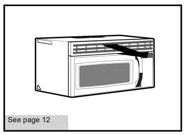
A Charcoal Filter Accessory Kit is required for the nonvented exhaust. (See your Owner's Manual for the kit number.)
