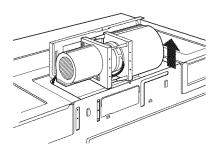
**4.** Remove the two screws holding the left side inlet sleeve to the blower unit. Snap the inlet sleeve off of the blower.
