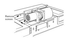
5. Roll the blower unit so that the right exhaust outlet faces the rear. Snap the inlet sleeve back onto the left side with the opening facing down. Note: The left side sleeve opening must always face downward. Reinstall the 2 screws holding the inlet sleeve to the motor assembly.
