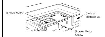
2. Open the blower motor by lifting it up at the back side of the microwave. Remove and save the top and back retaining screws that hold the blower motor in the microwave.
