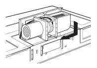
**7.** Secure the blower unit to the microwave with the two screws removed in Step 2.
