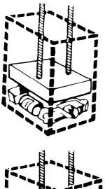
The compacting ram does not go to the drawer bottom. You will not see compacting of the first few loadings.
