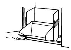
4. Hold Side-Lock Latch and tilt side of drawer until the latch clears the drawer front.
