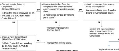
VCC Resistance Check Check resistance between terminals 1 and If all resistances are equal, compressor is operative
