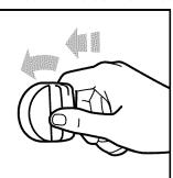
clockwise to the LIGHT position. The clicking sound is the ignitor sparking. Make sure the burner has lit.
