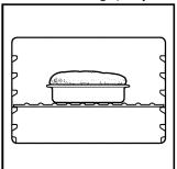
preheat conditioning time ends. During baking/roasting, the oven burner will turn on and off to keep the oven temperature at the setting.
