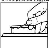
clean them with a straight pin. Do not enlarge or distort the port. Do not use a wooden toothpick. If the burner needs to be adjusted, call a qualified technician for service.
