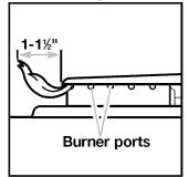
size and shape as shown. A good flame is blue in color. If the flames are not burning at all ports, you may need to clean the burner ports.
