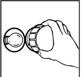
**3.** Remove the light bulb from its socket. Replace the bulb with a 40-watt appliance bulb.
