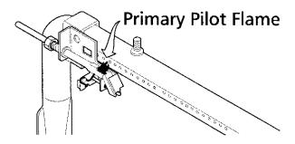
After 20-40 seconds, the main oven burner should ignite and burn until the oven temperature has reached 300°F. At that time, the oven pilot should get smaller, moving up away from the metal bulb which will turn off the main oven burner after 20-40 seconds.
