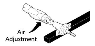
If the air is properly adjusted, the flame will be steady, relatively quiet, and have approximately 1/2" sharp blue cone. (Usually about the center of air shutter's ajustment.)
