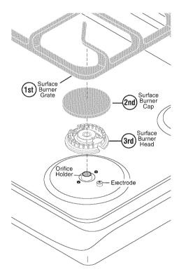
**To Remove and Replace the Surface Burner Caps and Burner Heads (all models) -** Remove in the following order: (1st) surface Burner Grates, (2nd) Burner Caps and (3rd) Burner Heads. Reverse the procedure above to replace the surface Burner Caps, Burner Heads and Burner Grates.
