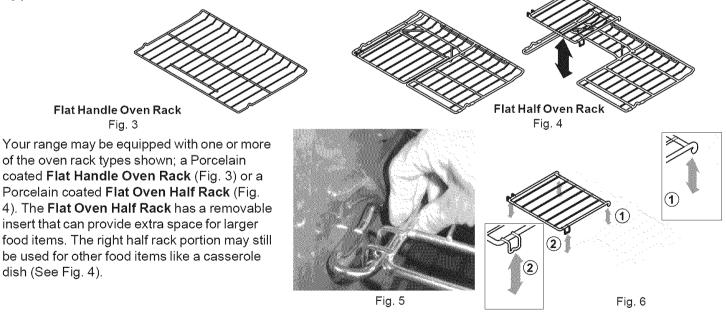
To remove the Half Oven Rack insert, squeeze on the left front insert side (See Fig. 5) of the rack and tilt out clockwise. To reinstall insert rear hooks at back of insert (See 1-Fig. 6) and lay insert down. Make sure both insert front hooks snap into rack (See 2-Fig. 6).
