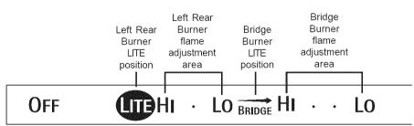
Fig. 3 - Left Rear Bridge Burner Surface Control Knob markings
