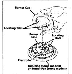
**ACAUTION** Use caution when replacing the burner cap so the electrode is not damaged. This may cause a delayed ignition or prevent the burner from igniting.
