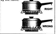
*For most cooking*, start on the highest control setting and then turn to a lower one to complete the process. Use the chart below as a guide for determining proper flame size for various types of cooking. The size and type of utensil used and the amount of food being cooked will influence the setting needed for cooking.
