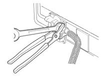
Use 15/16" combination wrench and channel lock pliers to attach the flexible connector to the adapters. Check that connector is not kinked.
