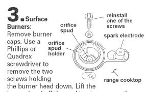
burner head off the cooktop to uncover the orifice spud holder. The orifice spud is recessed in the holder.
