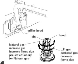
Oven burner: Use 1/2" combination wrench to loosen the orifice hood away from pin (approximately 2 to 2-1/2 turns). The burner flame cannot be properly adjusted if this conversion is not made.
