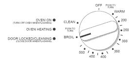
Push in and turn the oven selector control knob to "BROIL." If the burner fails to light due to air remaining in the gas line, reset the oven control by turning selector knob to "OFF" and then again to "BROIL".
