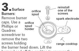
the burner head down. Lift the burner head off the cooktop to uncover the orifice spud holder. The orifice spud is recessed in the holder.
