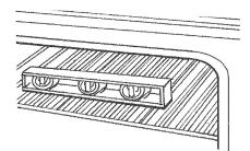
Place rack in oven. Place level on rack, first side to side; then front to back. If range is not level, pull range forward until rear leveling leg is removed from the anti-tip bracket. Use 3/8" drive ratchet and channel lock pliers to adjust leveling legs up or down until range is level. Push range back into position. Check that rear leveling leg is engaged in anti-tip bracket.
