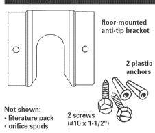
Bracket must be securely mounted to sub-floor. Thickness of flooring may require longer screws to anchor bracket to sub-floor. Longer screws are available from your local hardware
