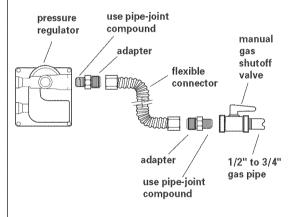
A 1/2" male pipe thread is needed for connection to pressure regulator female pipe threads.
