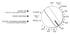
Push in and turn the oven selector control knob to "350°F." If the burner fails to light due to air remaining in the gas line, reset the oven control by turning selector knob to "OFF" and then again to "350 F".
