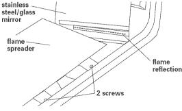
You can check the burner flame by removing the flame spreader or by using a mirror.
