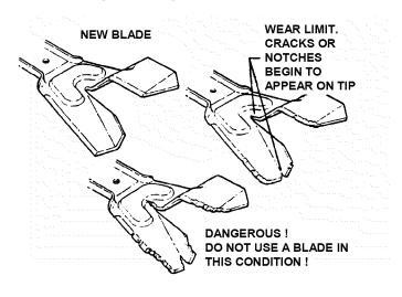
**2.** Replace the blade if it is badly chipped, bent, noticeably out of balance or has cracks or notch in either tip. See Figure 4.1 & 4.1A. Replace with new blade.
