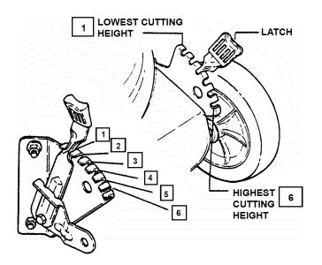
**2.** Set all wheels at the same cutting height. The highest cutting position is Notch 6. The lowest cutting position is Notch 1. See Figure 2.10.
