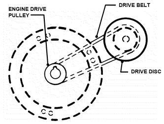
TOP VIEW OF STRETCH TYPE BELT ROUTING
