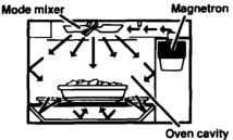
A magnetron in the microwave oven produces microwaves. The microwaves move into the oven where they are scattered or stirred by a mode mixer (like a fan). Microwaves bounce off metal oven walls and are absorbed by food.
