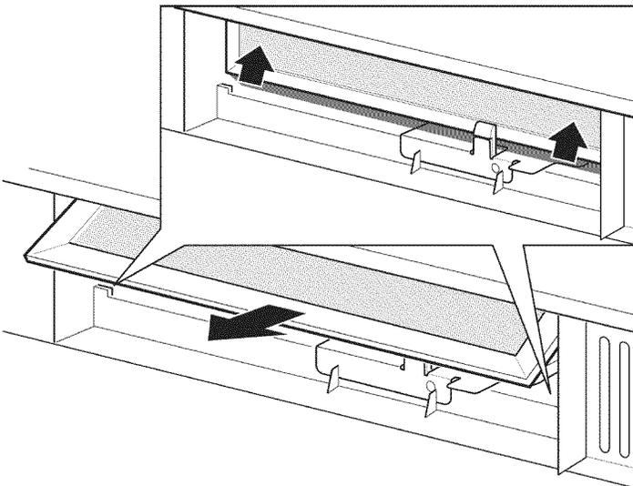
5. Open light cover located behind filter mounting by carefully pulling up on the front edge.
