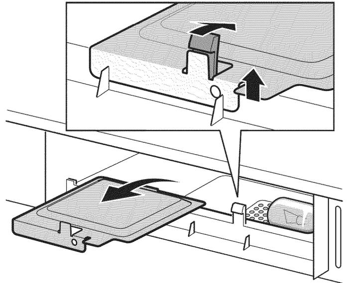
6. Remove old light bulb and replace only with equivalent 30 watt bulb available from parts distributor. Bulbs are also available at most hardware stores or lighting centers.
