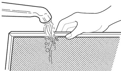
2. Soak the ventilation filters in hot water using a mild detergent. Rinse well and shake to dry. **Do not use ammonia or wash in a dishwasher. The aluminum on the filter will corrode and darken.**
