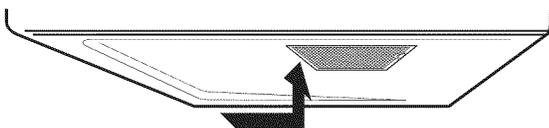
3. To reinstall the exhaust ventilation filter, slide it into the side slot, then push up and toward oven to lock. Reinstall the 2nd filter using the same procedure.
