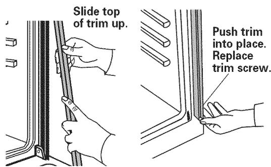
**7.** Slide top end of each trim upward onto oven side rails. Push each trim into place at bottom of trim. Use screws to attach each trim to oven. Take care not to scratch other surfaces with ends of trim.
