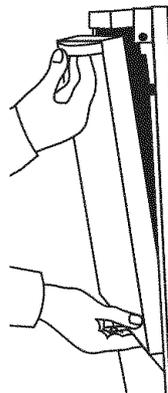
**2.** Completely open lower oven door. Insert small end of a door removal pin into each door hinge. Grasp door handle from the bottom and gently close door as far as it will shut. Lift slightly and grasp bottom of door with other hand. Pull door out at bottom to remove. Set door aside on protected surface. Repeat for upper oven door.
