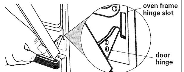
**9.** Replace the single or upper oven door by inserting ends of hinges into hinge slots in oven frame. Push behind each hinge so that hinges are pushed into oven frame as far as they will go. Open door and remove both door removal pins. Close and open door to check that door closes and opens completely. If door does not close or open completely, you have not pushed hinges completely into frame. Repeat door removal step and reinsert door into hinge slots again.
