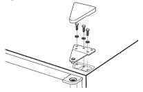
**NOTE:** When removing the door, watch for washer(s) between the center hinge and the bottom of the freezer door that may stick to the door. Do not lose.
