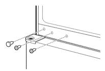
Install the center hinge designed for the left side that came with the refrigerator, with the screws, spacer and washer(s) (on some models) that you removed in Step 2.
