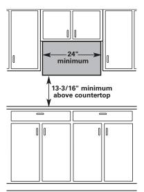
Note: This microwave oven is intended for installation over a countertop. Do not install this microwave oven above any heat source such as a range or cooktop.
