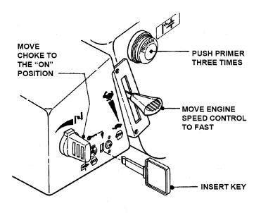
**5.** Push primer button three times to start a cold engine. **NOTE:** Do not use primer button to start warm engine. See Figure 2.4.
