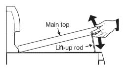
ACAUTION When lowering the lift-up range top, grasp the sides with finger-tips only. Be careful not to pinch fingers. DO NOT drop or bend the range top when raising or lowering. This could damage the surface.
