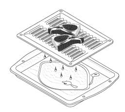
The broiler pan and the insert (some models) allows grease to drain and be kept away from the high heat of the broiler. **DO NOT** use the pan without the insert. **DO NOT** cover the insert with foil; the exposed grease could ignite.
