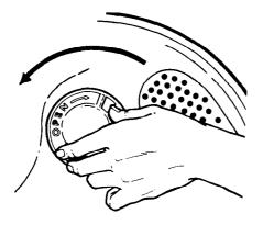
**4.** Replace the light bulb cover and turn it counterclockwise until it locks in place.
