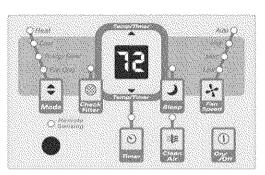
**Note:** Tap or hold either up ( $\blacktriangle$ ) or down ( $\forall$ ) button until the desired temperature is seen on the display. This temperature will be automatically maintained anywhere between 60°F (16°C) and 90°F (32°C) for cooling mode. The temperature will be automatically maintained anywhere between 55°F (13°C) and 80°F (27°C) for heating mode. If you want the display to read the actual room temperature. See "To Operate on Fan Only" section on Page 7.
