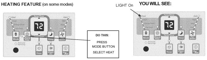
**Note:** This feature can be used with any combination of FAN Speeds(Low speed only on 115V models), Timer, or Sleep Modes. When in the "Heat" Mode, the fan will run continuously while heat is needed. The temperature will automatically be maintained anywhere between  $55^{\circ}$  F( $13^{\circ}$ C) and  $80^{\circ}$  F ( $27^{\circ}$ C) When the room set temperature is satisfied, the fan will cycle off and on to circulate and sample the room air.
