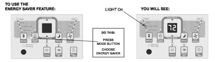
Note: In this mode, the fan will continue to run for another 3 minutes after the compressor shuts off. The fan then cycles on for 2 minutes at 10 minute intervals until the room temperature is above the set temperature, at which time the the cooling system turns back on.
