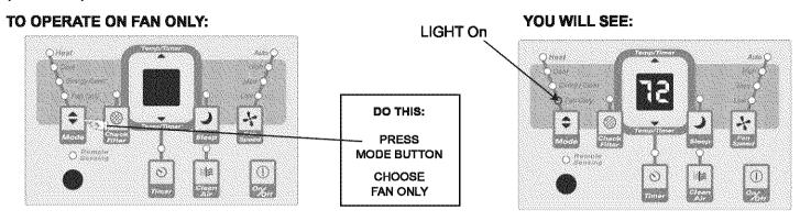
Note: Use this function only when cooling is not desired, such as for room air circulation or to exhaust stale air. (Remember to open the vent during this function, but keep it closed during cooling for maximum cooling efficiency.) You can choose any fan speed you prefer. (Except "Auto Fan").
