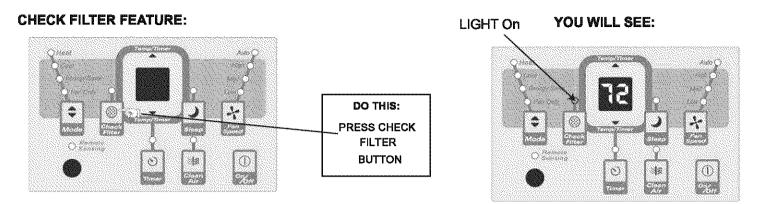
Note: This feature is a reminder to clean the Air Filter (See Care and Cleaning) for more efficient operation and cooling. The LED (light) will illuminate after 250 hours of operation. To reset after cleaning the filter, press the "Check Filter" button and the light will go off.
