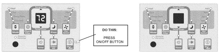
**Note:** When unit is shut off in the Heat Mode, the fan will continue to run for a few seconds to dissipate residual heat within the unit.
