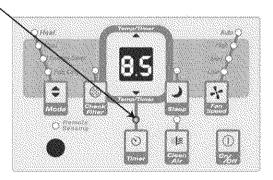
Note 1: For Delay Stop, the unit must be in the On position. Note 2: For Delay Start, the unit must be in the Off position. First, PRESS TIME BUTTON
