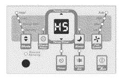
If the display reads"HS", a sensor has failed.
