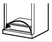
**3.3** Remove the tape and tilt the door away from the cabinet. Lift the door from the pin in the bottom hinge bracket. (If the plastic washer sticks to the door bottom, put it back on the hinge.)
