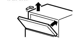
6.2.3 Make sure the door is slightly above the top of the cabinet and the gap between the doors is even across the front. Tighten the top hinge screws. Do not overtighten these screws—tighten them until they are just snug, then turn them another one-half turn.
