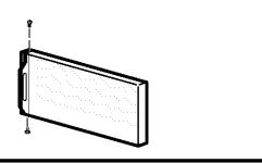
**5.4.3** Remove the screw from the right top edge of the door and insert it into the handle screw hole on the left side.
