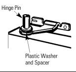
6.1.3 Tilt the door toward the cabinet. As the door is brought into position, slide the hinge under the head of the screw which earlier had been partly driven into the outermost hole. Insert the remaining screw, then tighten both screws securely.
