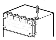
2.3 Lift the hinge (and the shim glued to it) straight up to free the hinge pin from the socket in the top of the door and set it aside, along with its screws.
