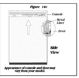
6. Unlatch door and open while supporting outer door on both sides at bottom to keep in place. Align screw holes and replace
