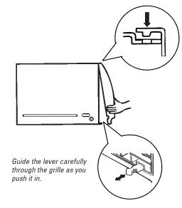
**D** Lift the inlet grille and secure the front frame with a type A screw through the front grille. Lower the inlet grille back into place.
