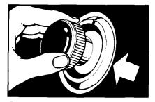
C. Start the washer by pulling out the Control Knob. The washer will fill to the selected water level with the selected wash water temperature. After filling, the washer will agitate for the selected number of minutes.
