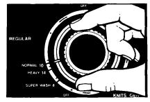
**B.** Stop when the indicator on the knob's outer ring points to the number in the wash cycle you want. The numbers are minutes of wash time.
