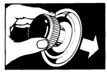
D. To stop the washer at any time, push in the Control Knob. To restart the washer, pull out the Cycle Control Knob.
