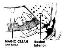
The lint filter at the bottom of the washer basket cleans itself. During agitation, wash and rinse water pass over the filter, separating lint from water. The collected particles of lint are then continuously spun away from the filter and washed out of the system at the end of the wash cycle.
