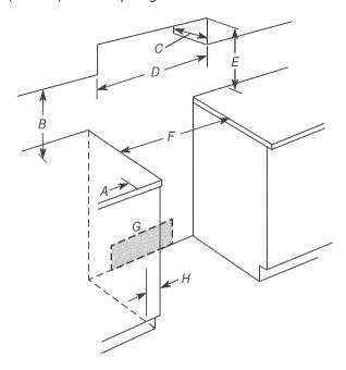
A. 4" (10.2 cm) min. clearance from both sides of range to side wall or other combustible material
