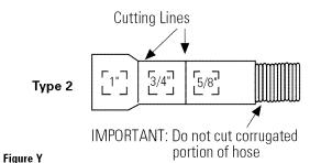
• If a longer drain hose is required, add up to 42" of length for a total of 10' to the factory installed hose. Use 5/8" or 7/8" inside diameter hose and a coupler to connect the two hose ends. Secure the connection with hose clamps.
