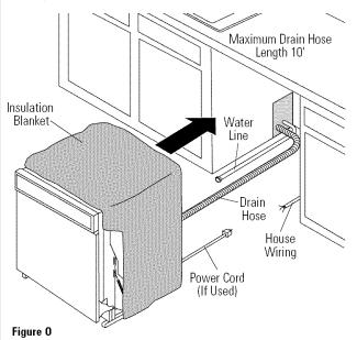
**Tip:** Position water line and house wiring on the floor to avoid interference with base of dishwasher.
