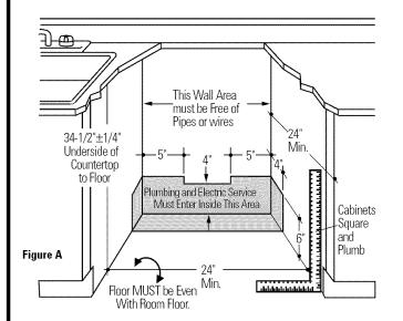
The rough cabinet opening must be at least 24" deep, 24" wide and approximately 34-1/2" high from floor to underside of the countertop.
