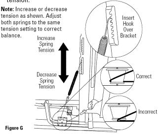
**Tip:** If door spring adjustment is necessary, check door opening and closing. If door does not open easily or falls too quickly, check spring cable routing. The cable is held in place by "shoulders" on the pulley. Check to be sure cable has not slipped over the pulley shoulders.
