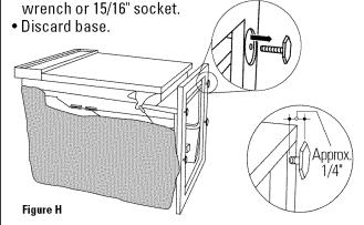
• Screw leveling legs back into the dishwasher frame, approximately 1/4" from frame as shown.
