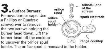
Note: Reinstall one of the screws through the range cooktop to hold orifice spud holder in place while removing and replacing orifice spuds.
