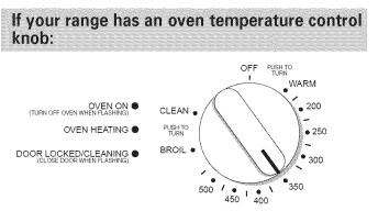
Push in and turn the oven selector control knob to "350". If the burner fails to light due to air remaining in the gas line, reset the oven control by turning selector knob to "OFF" and then again to "350".
