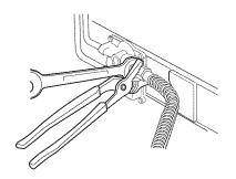
Use 15/16" combination wrench and channel lock pliers to attach the flexible connector to the adapters. Check that connector is not kinked.
