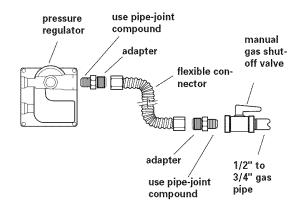
A 1/2" male pipe thread is needed for connection to pressure regulator female pipe threads.
