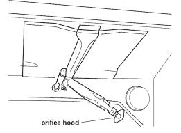
**D • Broil burner**: Use 1/2" combination wrench to turn the orifice hood down snug onto pin (approximately 2 to 2-1/2 turns). **DO NOT OVERTIGHTEN**. The burner flame cannot be properly adjusted if this conversion is not made.
