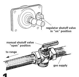
■ Check that range regulator shutoff valve is in the "on" position. Open the manual shutoff valve in the gas supply line.
