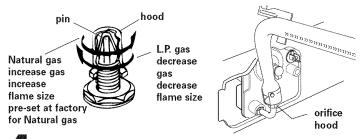
• Oven burner: Use 1/2" combination wrench to turn the orifice hood down snug onto pin (approximately 2 to 2-1/2 turns). DO NOT OVERTIGHTEN. The burner flame cannot be properly adjusted if this conversion is not made.
