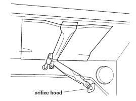
**D** ■ Broil burner: Use 1/2" combination wrench to loosen orifice hood away from pin (approximately 2 to 2-1/2 turns). The burner flame cannot be properly adjusted if this conversion is not made.
