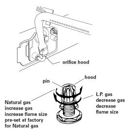
• Oven burner: Use 1/2" combination wrench to loosen the orifice hood away from pin (approximately 2 to 2-1/2 turns). The burner flame cannot be properly adjusted if this conversion is not made.
