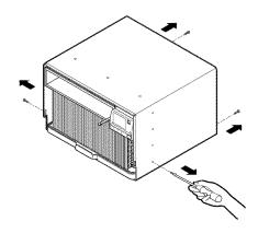
Slide the air conditioner from the case by gripping the base pan handle and pulling forward while bracing the case.
