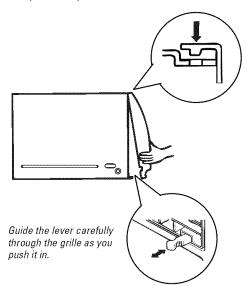
Lower the inlet grille and secure the front frame with a type A screw through the front grille. Raise the inlet grille back into place.
