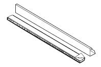
Install the top mounting rail with 3 type A screws on the inside of the case. Insert the frames for the accordion panels into the top mounting rail and the frame guides. Attach the accordion panels to the side of the case using 4 type A screws on each side.
