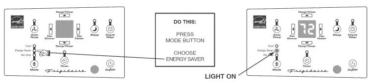
**Note:** In this mode, the fan will continue to run for another 3 minutes after the compressor shuts off. The fan then cycles on for 2 minutes at 10 minute intervals until the room temperature is above the set temperature, at which time the the cooling system turns back on.
