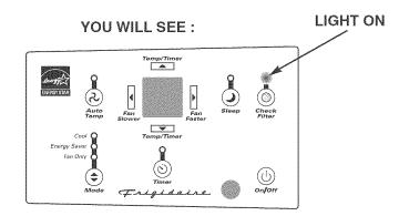
**Note:** This feature is a reminder to clean the Air Filter (See Care and Cleaning) for more efficient operation and cooling. The LED (light) will illuminate after 250 hours of operation. To reset after cleaning the filter, press the "Check Filter" button and the light will go off.
