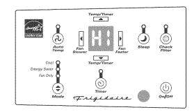
Press the Fan Faster button will increase the fan speed from Low (LO), to Medium (ME), to High (HI). The digital display will indicate your chosen speed. Press the Fan Slower button will decrease the fan speed from High (HI), to Medium (ME), to Low (LO). The digital display will indicate your chosen speed. After 5 seconds the display will revert back to the set temperature.
