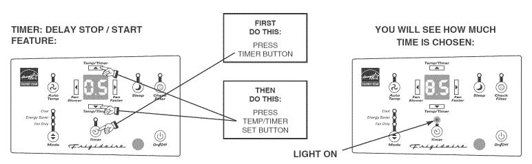
**Note 1:** For Delay Stop, the unit must be in the On position. **Note 2:** For Delay Start, the unit must be in the Off position.
