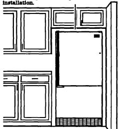
The refrigerator can be flush against the back wall
