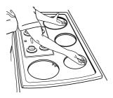
**3.** To open, grip the left and right front element openings and lift. The support rod will swing forward. Pull the rod until it rests at the front edge of the burner box.
