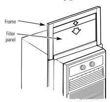
Insert the filler panel frame over the filler panel and into the side guides.
