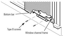
Make sure the air conditioner is firmly anchored to the window channel frame.
