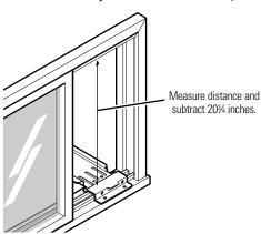
Insert the uncut end of the filler panel into the top guide. Center the filler panel side-to-side in the top guide.
