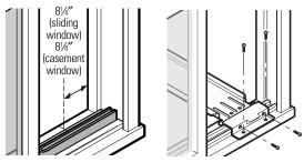
Pull the support angle against the outside wall and tighten the screws on top of the support platform. Adjust the leveling bolt so the support platform is installed with a slight tilt to the outside. Use a level; about 1/3 bubble will be the correct slant to the outside. Tighten the nut.
