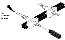
Test to verify if "LOW" setting should be adjusted
