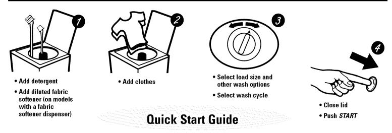
NOTE: When making a selection with any knob, simply point the knob anywhere within the shaded range for that setting.
