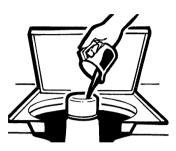
*The agitator cap* fits into the top of the agitator. If it accidentally comes off, simply put it back on.
