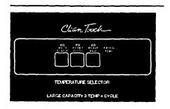
Press a temperature selection which matches the type of fabric being dried. The indicator will appear over the temperature selection you have chosen.
