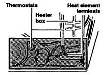
Electric dryer with back panel removed
