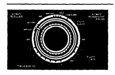
Select a cycle by turning the Cycle Control Knob either way. Stop when the indicator on the knob's outer ring points to the cycle and setting you want. See pages 6-7 for further cycle information.
