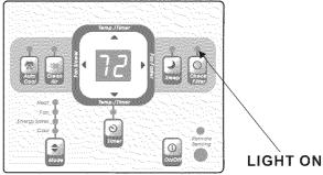
NOTE: This feature is a reminder to clean the Air Filter (See Care and Cleaning) for more efficient operation. The LED (light) will illuminate after 250 hours of operation. To reset after cleaning the filter, press the "Check Filter "button and the light will go off.
