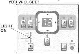
NOTE: In this mode, the fan will continue to run for 3 minutes after the compressor shuts off. The fan then cycles on for 2 minutes at 10 minute intervals until the room temperature is above the set temperature, at which time the compressor turns back on and cooling starts.
