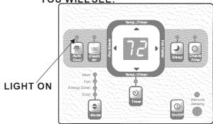
NOTE: Fan starts at High Speed and adjusts to a slower speed as the room temperature dictates. For example if the room does not get too warm, it will stay at the slowest speed. If the room temperature rises quickly, such as a door being opened, it will automatically go to the highest speed. The fan speeds will re-adjust back to the slowest speed as the room returns to the original set temperature. Press either the fan slower or fan faster button to adjust the fan speed manually.
