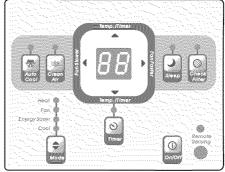
A 2 Digit Display is used to indicate the Fan Speed setting, from 10 through 99. When the " SLOW" button is pressed, the motor  $\,$ speed will slow down at multiple intervals (90 distinct settings), to a minimum setting of 10. To speed the motor up, press the "FASTER" button. The speed will increase at multiple intervals to a maximum setting of 99. After 5 seconds the control will automatically change back to displaying the set temperature.
