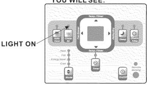
NOTE: When this feature is "ON", the electronic air purifier is energized to remove pollen and impurities from the air. To cancel this feature, press the Clean Airbutton (the LIGHT will turn off).
